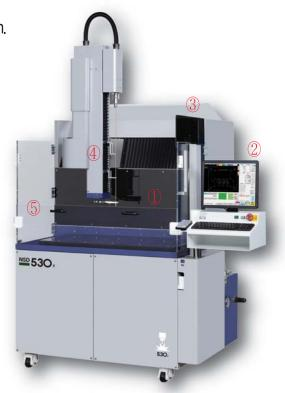
▼ 3 stage fine discharge control for stable drilling (Normal EDM drillers use 1 stage discharge control)
